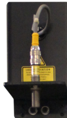
Laser Pointer Allows operator a visual indicator for plate alignment and torch positioning.
